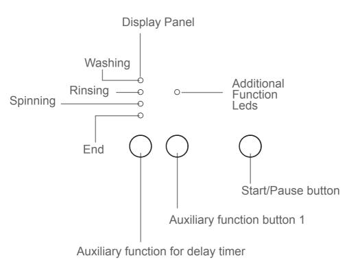
From the function leds of your machine, you can see how much longer it will start to run after, the auxiliary functions you have selected and the stage of the programme you are running on your machine. (U pre wash / wash state, ) rinsing stage, () spinning stage).
