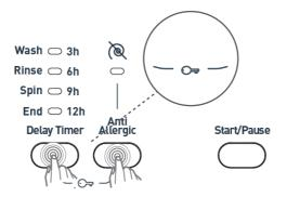
If pressed any button while child lock is active, the Additional Function Leds will blink on the display.
