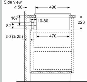
When installing directly against outer walls that are not insulated ( $\mu \geq 0.5 \text{ W/m}^2 \cdot \text{°C}$ ), we recommend using partially or fully ducted recirculation configurations.
