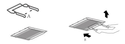
Please use both hands to hold the holding parts(A). Then move it along the direction B until it reaches the position like the picture showing. Finally, lift the racks up to move.
