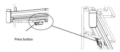
Press the front clip button to remove the boss off the outer wire.
