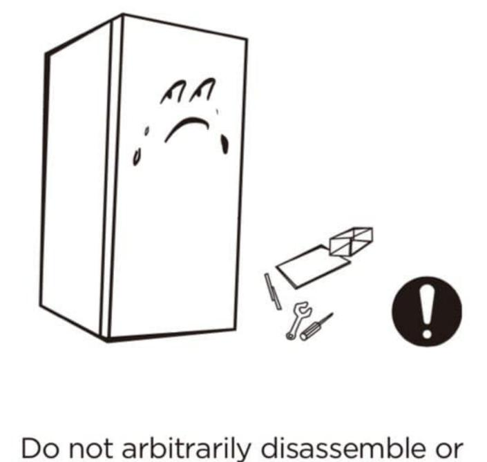
reconstruct the refrigerator, nor damage the refrigerant circuit; maintenance of the appliance must be conducted by a specialist.
