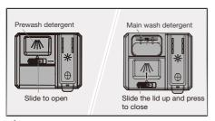
If powder or liquid dishwasher detergent is used, add a small amount of the detergent to the compartment for prewash detergent.
