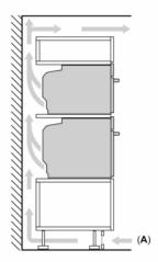
If the appliance will be installed underneath a hob, the following worktop thicknesses (including substructure if necessary) must be taken into account.
