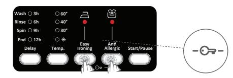
If pressed any button while child lock is active, the Additional Function Leds will blink on the display.
