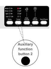
You can gradually decrease the washing water temperature between the maximum washing water temperature of the selected programme and cold washing \*\* selections by pressing temperature adjustment button.
