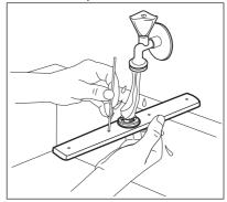
4. To install the spray arm back, insert the mounting element in the spray arm and fix it in the duct by turning it counterclockwise. Make sure that the mounting element locks into place.
