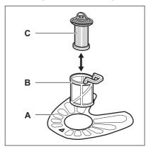
Turn the filter (B) counterclockwise and remove it.
