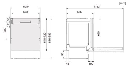
\*Remove the plastic strips if the recess dimension is 596-598 mm. Exercise caution! The edges may be sharp. Wear protective gloves!
