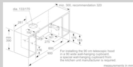
For installing the 90 cm telescopic hood in a 90 wide wall-hanging cupboard, a special wall-hanging cupboard from the kitchen unit manufacturer is required.
