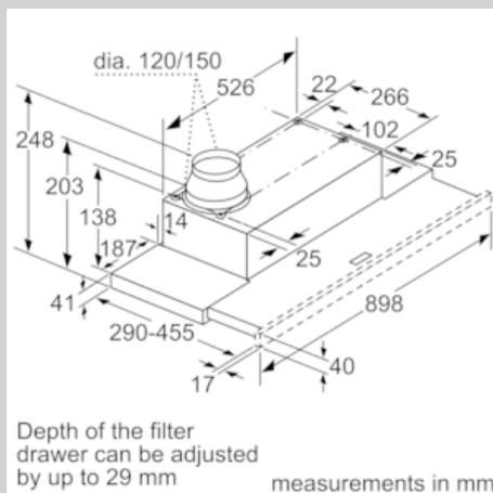
Depth of the filter drawer can be adjusted by up to 29 mm
